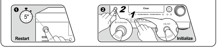
Try restarting the unit. Switch this unit to standby, then do **1**. If the problem is not fixed, try the following: • Unplugging the power cord and HDMI cables then replugging them in again • Initializing the settings (do **2** while this unit is ON)
