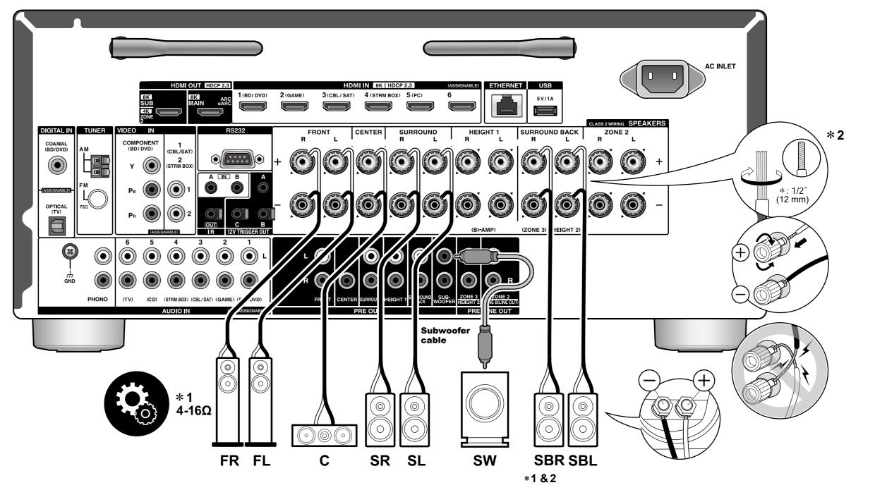
Connect speakers with 4  $\Omega$  to 16  $\Omega$  impedance. Twist the ends of the speaker cable wires tightly.
